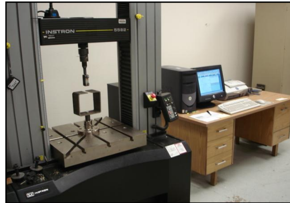
Figure 6: Expanded view of fastener withdrawal test setup, including Instron test workstation.
