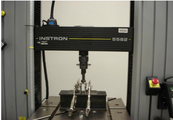
Figure 4: Bend-yield test setup in Instron tensile machine, expanded view
