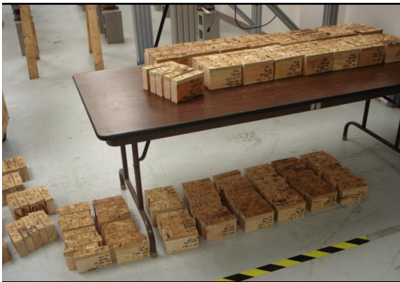
Figure 7: Fastener withdrawal specimens, prepped and awaiting testing
