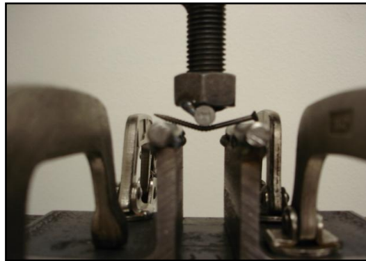
Figure 3: Bend-yield test specimen at ultimate load
